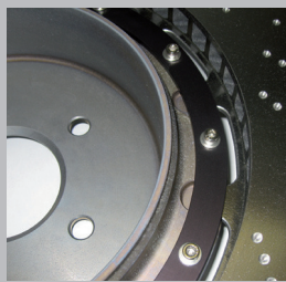
Rear disc with integral drum
